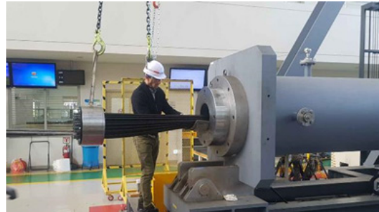
Fig. 22. Cable anchorage watertightness test (Posco)
