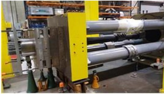
Fig. 21. Cable anchorage fatigue test (CTL Group)
