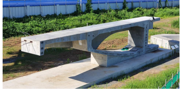
Fig. 18. Reinforcing girder mock-up test
